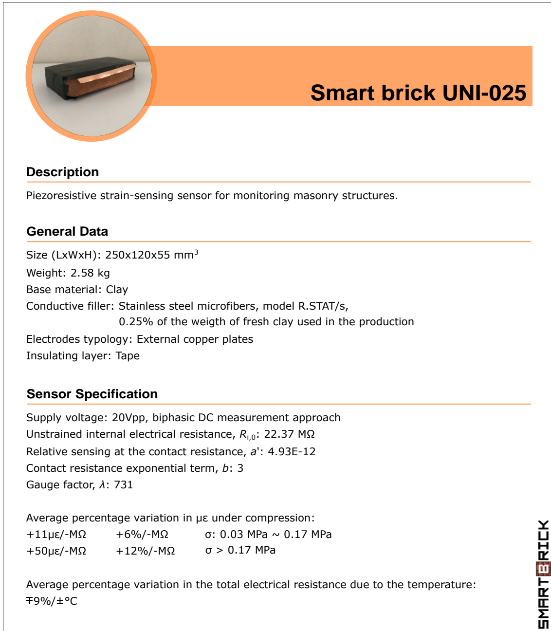
Fig. 4.30: Conceptual exemplification of the data sheet of a smart brick.
